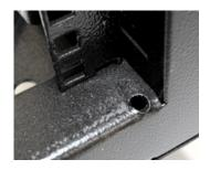
Locate the mounting holes on the side you wish to hang the door and insert the mounting guides [F], there will be one at the top and one at the bottom.
