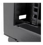
Inserting the Cage Nuts for the Door Stops
