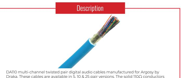
DA110 multi-channel twisted pair digital audio cables manufactured for Argosy by Draka. These cables are available in 5, 10 & 25 pair versions. The solid 110 $\Omega$  conductors are suitable for IDC punch down applications, therefore making it the ideal solution for jackfield to Krone applications. All sizes have blue LSOH jackets as standard and are supplied on 500m drums.
