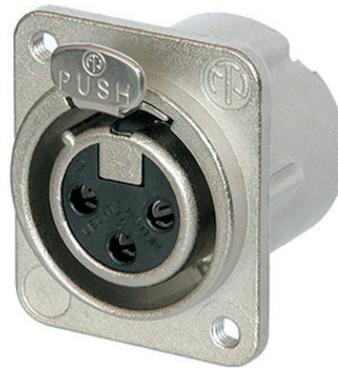
The Neutrik NC3FD-LX-M3 is a 3 pole female receptacle with solder cups, nickel housing, silver contacts and M3 mounting holes.
