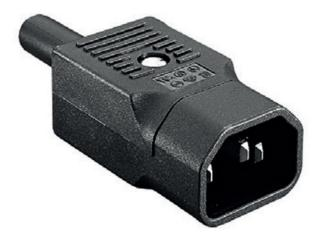
The Bulgin PX0686 (straight male connector) is a cable-mounting IEC power connector ideal for industrial applications, power management, and portable devices. Features include a black, straight male connector with rewireable screw terminals, nickel-plated brass contacts, and contact resistance of  $10m\Omega$ .
