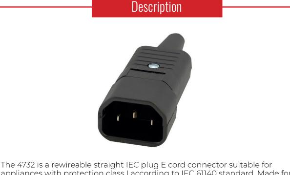
appliances with protection class I according to IEC 61140 standard. Made for appliance inlets with Pin temperature of 70°C, the maximum wire size is 3 x 1mm<sup>2</sup> (3 x 18AWG), and the maximum cable diameter of 8.5mm.
