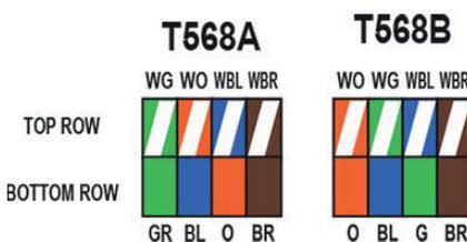
Align wires according to Termination Pattern either Type A or Type B.
