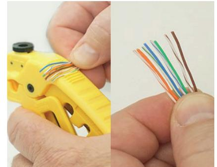
Straighten each wire conductor.
