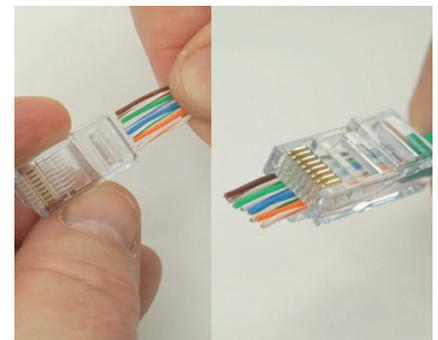
Hold the RJ45 plug upside down (strain relief clip facing down). Insert the wires into the back of the plug until they come out the front of the plug at least 1/2 inch (1.27cm).
