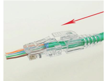
If using strain relief/boot, slide the boot up and into the back of the plug until the boot clip covers the top of the plug clip.
