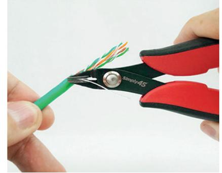
Trim off the "rip cord" at the cable jacket using Simply45 Flush Cutter (Part No: ME-99-008).
