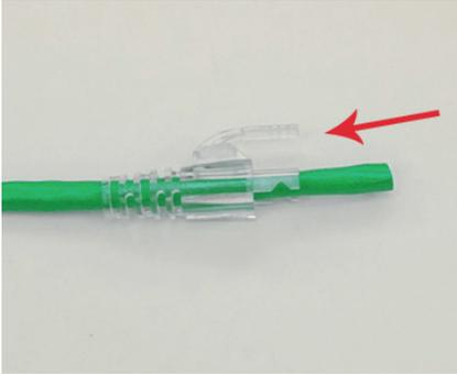
If using strain relief/boot, insert the boot onto the cable as shown.
