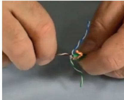
Separate each wire pair by untwisting.
