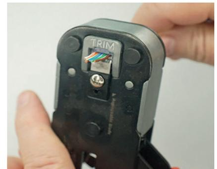
With one hand, firmly without stopping, compress the crimper handles all the way down in one steady non-stop motion.
