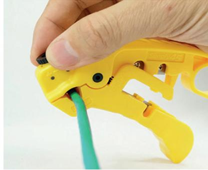
Using the Adjustable Cable Stripper (Part No: MC-99-9950), strip back the cable jacket about 1.5 inches (3.8cm).
