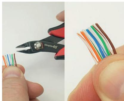
Using a flush cutter, trim the wires straight across so all of the wires are the same length.
