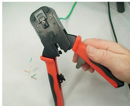
If the crimper handles do not release this means that you have not completed the crimping cycle. Simply squeeze the crimper handles further down until the crimper handles release.
