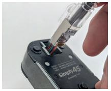
Insert the plug into the crimping socket on the S45-C100/S45-C101 Simply45 pass-through crimper. (Part No: ME-99-008).
