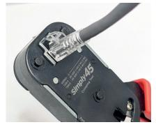
Make sure plug goes completely inside the crimping socket.
