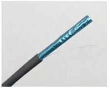
Be sure not to nick the wire insulation. If you nick the wire insulation, cut the cable off for all exposed wire cable pairs and re-strip the cable.
