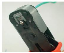
The Simply45 crimper is a ratcheted crimper. The crimper will not open up until the crimping process has been fully completed. This assures that the wire trims and pin sets have been done correctly.
