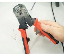
If the crimper handles do not release this means that you have not completed the crimping cycle. Simply squeeze the crimper handles further down until the crimper handles release.
