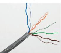
Separate each wire pair by untwisting. Push the drain wire back.
