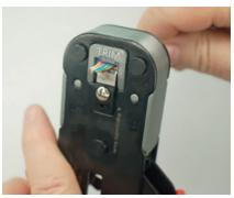
With one hand, firmly without stopping, compress the crimper handles all the way down in one steady non-stop motion.
