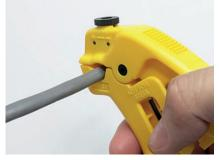
Using the Adjustable Cable Stripper (Part No: MC-99-9950), strip back the cable jacket about 1.5inches (3.8cm).
