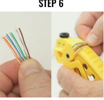
Straighten each wire conductor. Hint: Use wire straightening comb on top of Adjustable Stripper for faster straightening and less finger fatigue.
