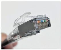
Then remove the terminated RJ45 plug from the crimping socket. Quickly inspect that all wires have been closely trimmed to the plug in the front.
