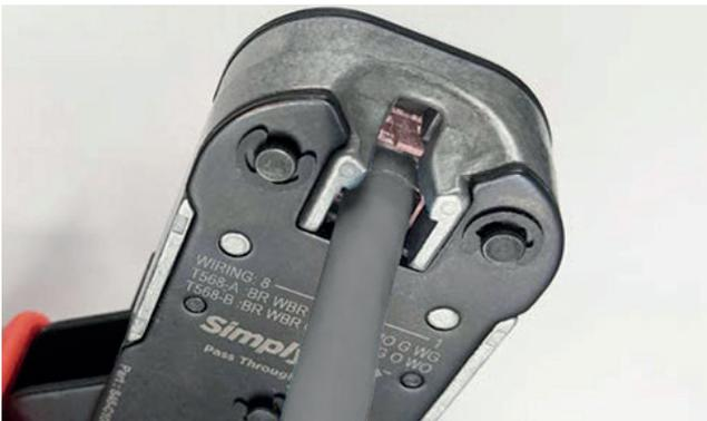
Insert the loaded plug into the Simply45® Heavy Duty RJ45 Crimper Tool (Part No: MA-99-9951). Make sure to completely insert the plug into the crimper socket.
