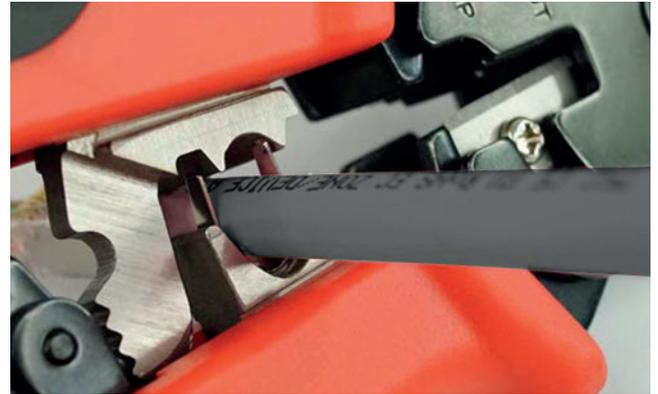
Using the external ground arm crimp feature on the Simply45 Shielded External Ground Crimper (Part No: MA-99-9951), crimp the external ground wings until securely folded around the cable jacket.
