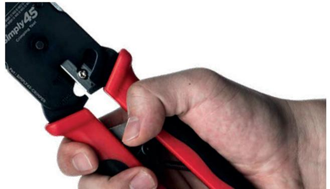
Compress the crimper handles all the way down with one swift and firm motion until the handles release.
