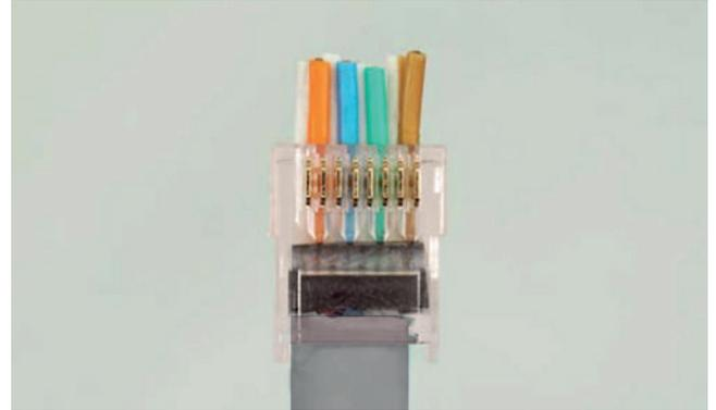
Insert the cable with the Bar45® into the plug allowing the wires to come out through the front of the plug as shown above. The S45-1750P plug is designed to accommodate the insertion of large diameter cables up to 8.0mm (0.315"). Work the cable jacket into the plug until fully inserted. Looking from underneath the plug, the cable jacket should meet or come close to the horizontal line (see above). Make sure the drain wire remains straight down the cable jacket.
