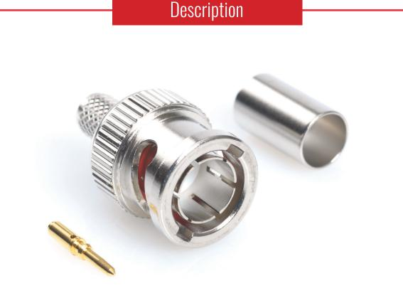
BNC True 75 ohm straight crimp plug, for applications up to 3GHz. Contact and crimp sleeve are annealed to provide a robust and durable termination, centre contact is gold plated. Suitable for Belden 1505A or Image 720 cables.
