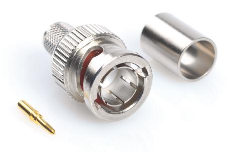
BNC True 75 ohm straight crimp plug, for applications up to 4.5GHz. Contact and crimp sleeve are annealed to provide a robust and durable termination, centre contact is gold plated. Suitable for Belden 1694A or Image 1000 cables.
