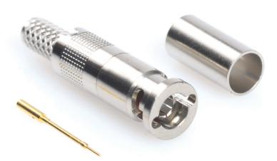
Micro BNC 75 ohm straight crimp plug. This true 75 ohm plug is designed for Full HD 1080p applications and general use up to 12GHz. With gold plated centre contact and annealed crimp zones these connectors offer a long term durable solution. Suitable Image 360 cable.
