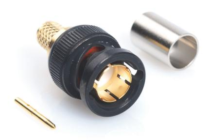
High Performance 12GHz True 75 ohm BNC with black finished body and gold plated inner and outer contact. High Performance 75 ohm BNC crimp plug Using standard US Crimp sizes tested to meet the requirements of SMPTE ST 2081-1 & ST 2082-1 for use in 6G & 12G systems. Suitable for Image 1000 cable.
