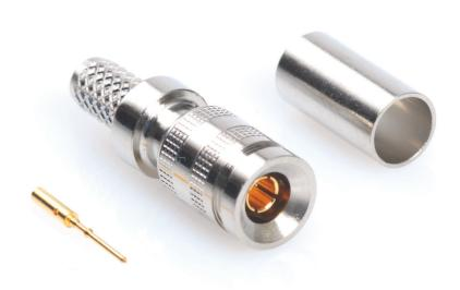
1.0/2.3 straight full crimp plug with gold plated centre and outer contact. Centre contact and crimp sleeve are annealed for enhanced performance. Suitable for Image 360 cable.
