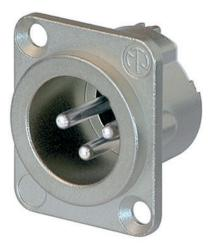
The Neutrik NC3MD-LX-HA is a 3 pole male receptacle with crimp termination (Standard B-Crimp), nickel housing and silver contacts.
