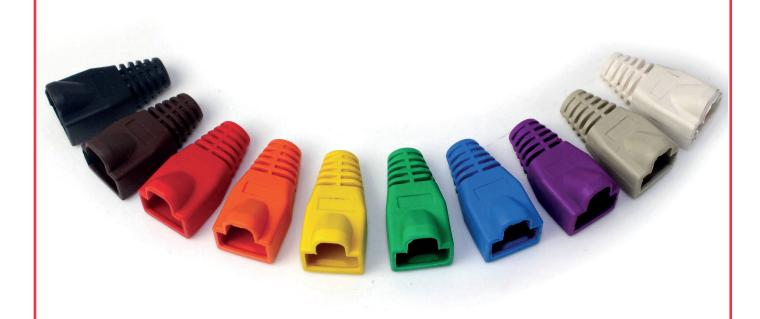
These durable RJ45 strain relief boots are perfect for Structured wiring cables with an overall diameter of 6mm. They prevent damage when fitted around RJ45 modular plugs providing effective strain relief by controlling the bend radius of the cable when the cable is connected, and protect the connector latch from snagging and subsequent damage.
