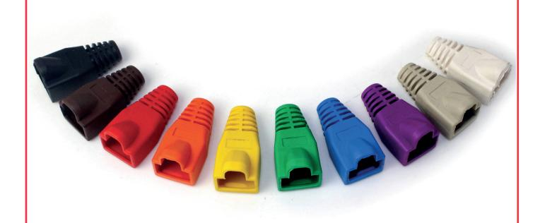
These durable RJ45 strain relief boots are perfect for Structured wiring cables with an overall diameter of 6.5mm. They prevent damage when fitted around RJ45 modular plugs providing effective strain relief by controlling the bend radius of the cable when the cable is connected, and protect the connector latch from snagging and subsequent damage.
