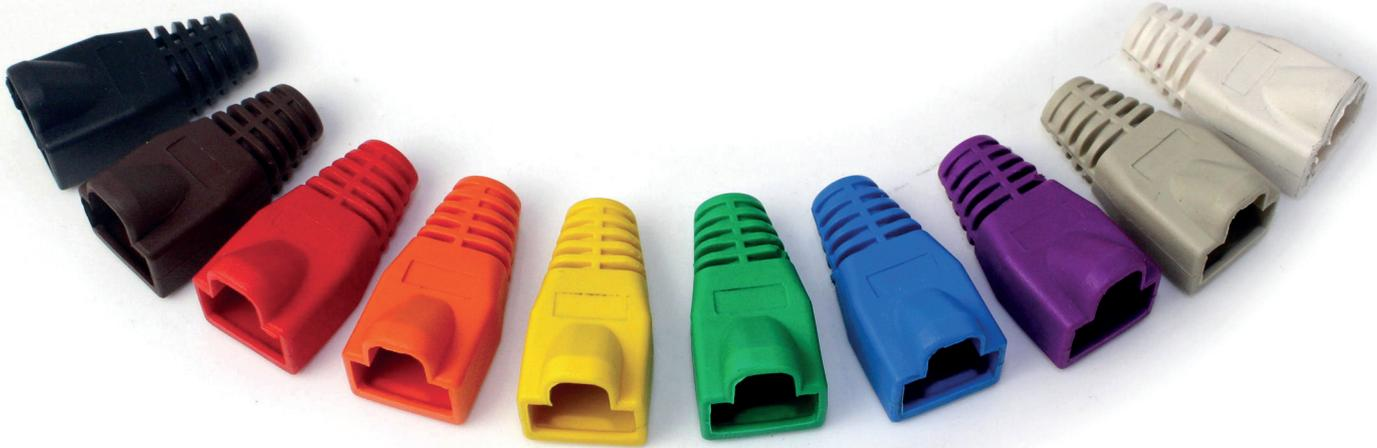
These durable RJ45 strain relief boots are perfect for Structured wiring cables with an overall diameter of 6.5mm. They prevent damage when fitted around RJ45 modular plugs providing effective strain relief by controlling the bend radius of the cable when the cable is connected, and protect the connector latch from snagging and subsequent damage.
