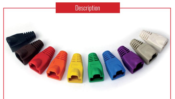
These durable RJ45 strain relief boots are perfect for larger OD Structured wiring cables with a diameter of 8mm. They prevent damage when fitted around RJ45 modular plugs providing effective strain relief by controlling the bend radius of the cable when the cable is connected, and protect the connector latch from snagging and subsequent damage.
