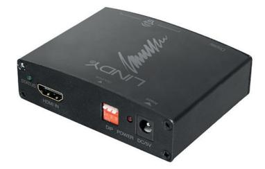
The Lindy HDMI 4K Audio Extractor is an effective solution for extracting audio from a HDMI source to both digital and analogue audio devices, while sending the video signal to a 4K display or projector. This is a perfect solution for connecting Non-HDMI AV receivers, or analogue 2-channel speaker setups to an HDMI source device, while also ideal for extracting audio and video to a display that requires separate speakers such as a PC monitor.
