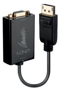
The Lindy DisplayPort 1.2 to VGA Converter is ideal for connecting a DisplayPort equipped source such as a PC or laptop to a VGA monitor. It supports high definition video resolutions up to 1920x1080@60Hz. Active conversion ensures compatibility with various graphics cards including AMD Eyefinity, NVIDIA surround and Intel Collage.
