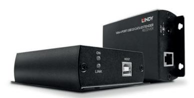
The Lindy USB 2.0 Cat.6 Extender extends the distance between four USB peripheral devices and a PC over distances up to 140m using a single Cat.6 UTP or higher network cable. Cat.5e UTP/STP cable can be used in lengths up to a maximum of 120m. For best performance and compatibility, we recommend the use of solid core patched cables. For best performance and compatibility, we recommend the use of solid core patched cables.
