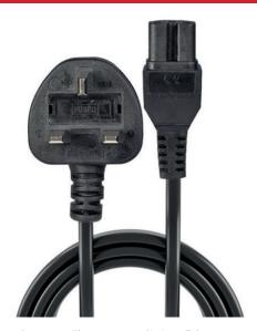
Note: These cables are referred to as "hot condition" because they are designed to be used with appliances that operate with temperatures of 120 degrees. They are similar to a C13 except they have a ridge opposite the earth pin.
