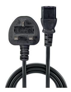
Note: Cables with IEC C13 sockets such as this are sometimes known by the generic term 'kettle lead'. Even though this term is commonly used, technically it is incorrect as a kettle requires special IEC C15/16 connectors rated at 120 degrees. So, although they look similar, a 'real' kettle lead features a connector with a cut out on the top. Standard IEC C13 cables cannot be plugged into kettles!
