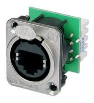
The Neutrik NE8FDV-YK is a panel mount receptacle with IDC punch down terminals, D-sized metal flange with latch lock, max. panel thickness 4 mm, mounting screws included.
