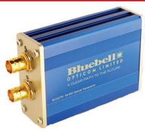
The BC323 is a Transceiver module for the conversion of an 3G-SDI, HD-SDI, SD-SDI and ASI signals into fibre optical cable, and another separate fibre signal to electrical signal.. Each incoming signal is auto-sensed and then equalised and reclocked prior to conversion and transmission down a separate single optical fibre/BNC.
