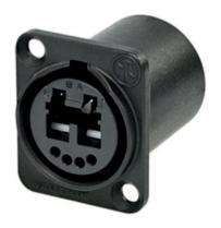
The Neutrik NO2-4FDW-A is a chassis connector with black chromium plating, 4 solder contacts and 1 LC-Duplex feedthrough socket, waterproof acc. to IP65 ingress protection in mated condition with SCDP-\*.
