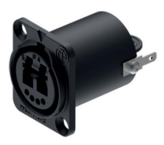
Neutrik NO2-4FDW-1-A is a chassis connector with black chromium plating, 4 solder contacts, 1 LC-Duplex feedthrough socket and 1 shell ground contact (for SMPTE cable shield), waterproof acc. to IP65 ingress protection in mated condition with SCDP-\*.
