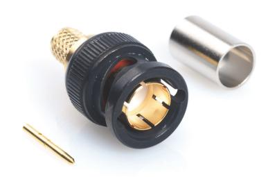
COAX Connectors "KORUS" Range of Ultra HD 12GHz True 75 ohm BNC's with black finished body and gold plated inner and outer contact. High performing BNC crimp plugs tested to meet the requirements of SMPTE ST 2081-1 & ST 2082-1 at 6G & 12G systems for use with the Argosy Image ULTRA Coax cable range.
