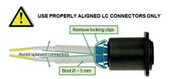
Avoid splayed connectors by using LCs without anti-snag collars and a boot diameter < 5 mm
