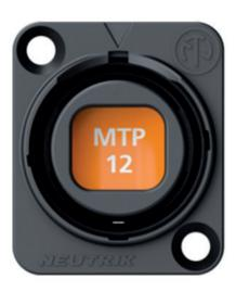
Neutrik NO12FDW-A has rear compatibility of opticalCON MTP® chassis fitting with standard MTP® (ELITE male) breakout cable allows easy adaptation to fibre standard connectors such as LC, SC, ST. The approved dust shutter ensures high mating cycles and minimal maintenance.
