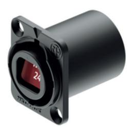
Neutrik NO24FDW-A has rear compatibility of opticalCON MTP® 24 chassis fitting with standard MTP® 24 (ELITE male with 20 N springforce) breakout cable allows easy adaptation to fibre standard connectors such as LC, SC, ST. The approved dust shutter ensures high mating cycles and minimal maintenance.
