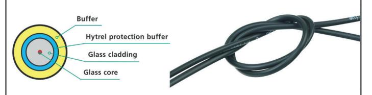
Conventional patch cables are sensitive in terms of undercutting the minimum bending radius and lateral pressure. Neutrik's tactical patch cables feature unique fibre design including a protection buffer which allows bendings with minimal radius and increased lateral pressure. Therefore the tactical patch cables are the right choice for permanent or semi-permanent applications.
