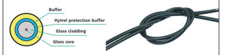
Conventional patch cables are sensitive in terms of undercutting the minimum bending radius and lateral pressure. Neutrik's tactical patch cables contain a unique fiber design including a protection layer which allows bending with minimal radius and increased lateral pressure. Therefore the tactical patch cables are the right choice for permanent or semi-permanent applications.
