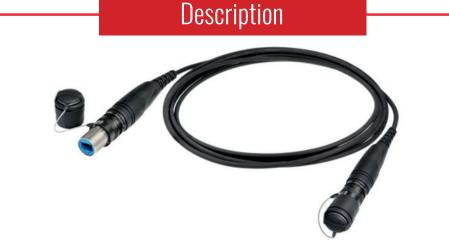
The Neutrik opticalCON DUO ADVANCED is an assembled 2 fibres rugged and lightweight mobile field cable, excellent cable retention due to aramid yarn, black PUR outer jacket, available in multi- and single mode (PC or APC), military approved. Ideal for audio and broadcast networks.
