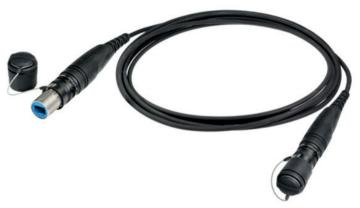
The Neutrik opticalCON DUO ADVANCED is an assembled 2 fibres rugged and lightweight mobile field cable, excellent cable retention due to aramid yarn, black PUR outer jacket, available in multi- and single mode (PC or APC), military approved. Ideal for audio and broadcast networks.
