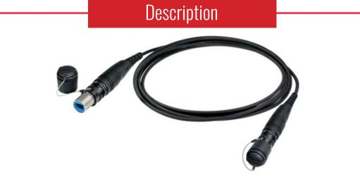
The Neutrik opticalCON DUO ADVANCED is an assembled 2 fibres rugged and lightweight mobile field cable, excellent cable retention due to aramid yarn, black PUR outer jacket, available in multi- and single mode (PC or APC), military approved. Ideal for audio and broadcast networks.
