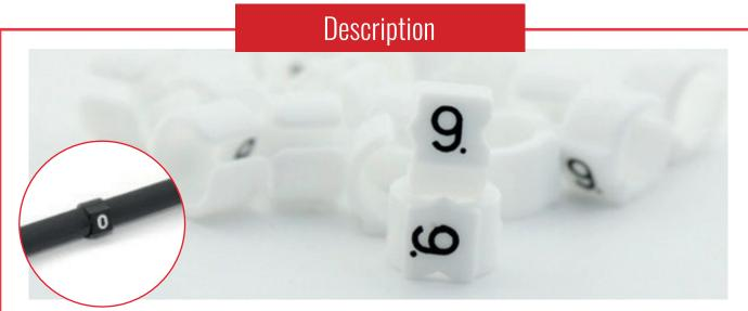
PS15 clip ident markers are fitted around a cable before or after termination or connector fitting. The markers' small profile allows them to be fitted on closely bunched wires on terminal blocks after termination. Colour-coded according to size for easy identification, the markers have a small chevron 'pip' on each side to ensure neat alignment when fitted.
