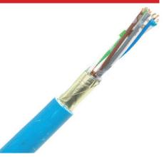
DA110 multi-channel twisted pair digital audio cables manufactured for Argosy by Draka. These cables are available in 5, 10 & 25 pair versions. The solid  $110\Omega$  conductors are suitable for IDC punch down applications, therefore making it the ideal solution for jackfield to Krone applications. All sizes have blue LSOH jackets as standard and are supplied on 500m drums.
