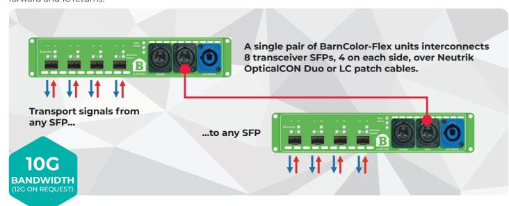
Insert any SFP and the signal will be converted and merged into the signal-stream along with all other signals from this and other cascaded units.
