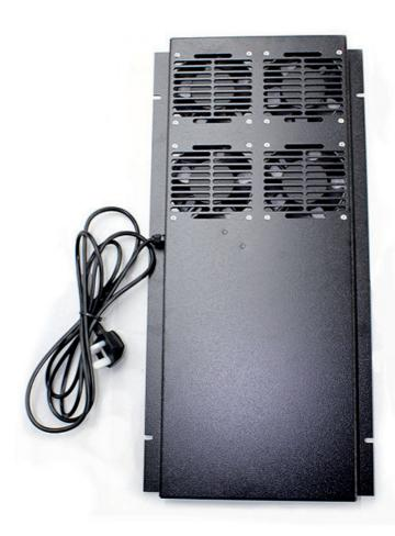
The Argosy 4 way IMAGE Rack fans are installed in the rack roof, for use for individual racks that need air distribution or in addition to cold aisle systems to tackle hot spots forming in the upper part of the racks where power distribution units and network switches are located.
