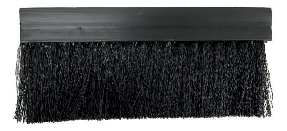
The Argosy 135mm brush is for installation in IMAGE rack lid knockouts. The brush sets are used when bringing cables from overhead into the rack. The brush stops foreign bodies from entering the internal rack space whilst supporting cables that transition from overhead. To install, the blanking plate is removed and brushed ipush fit either side of the opening.
