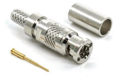
The High-Density BNC delivers true  $75\Omega$  ohm performance and is designed for applications where space is limited, such as racks with high cable counts and the latest large-generation digital routers. The High-Density BNC enables four times as many connections as the regular BNC, with a footprint that is 51% smaller than traditional BNC connectors and 40% smaller than the DIN 1.0/2.3.
