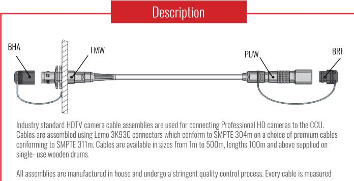
for insertion and return loss and consistently performs above industry standards. Additionally, all optical termini are 3D mapped and checked for conformance to EN 61300-3-23. Argosy is a certified Lemo termination partner.
