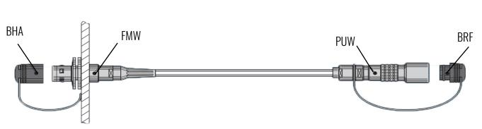
Industry standard HDTV camera cable assemblies are used for connecting Professional HD cameras to the CCU. Cables are assembled using Lemo 3K93C connectors which conform to SMPTE 304m on a choice of premium cables conforming to SMPTE 311m. Cables are available in sizes from 1m to 500m, lengths 100m and above supplied on single- use wooden drums.
