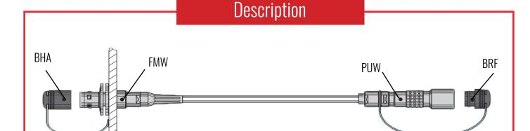
Industry standard HDTV camera cable assemblies are used for connecting Professional HD cameras to the CCU. Cables are assembled using Lemo 3K93C connectors which conform to SMPTE 304m on a choice of premium cables conforming to SMPTE 311m. Cables are available in sizes from 1m to 500m, lengths 100m and above supplied on single- use wooden drums.
