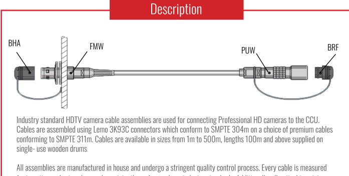
for insertion and return loss and consistently performs above industry standards. Additionally, all optical termini are 3D mapped and checked for conformance to EN 61300-3-23. Argosy is a certified Lemo termination partner.
