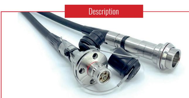
Industry standard HDTV camera cable assemblies are used for the connection of Professional HD cameras to the CCU. Cables are assembled using Lemo 3K93C connectors which conform to SMPTE 304m on a choice of premium cables conforming to SMPTE 311m.
