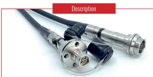
Industry standard HDTV camera cable assemblies are used for the connection of Professional HD cameras to the CCU. Cables are assembled using Lemo 3K93C connectors which conform to SMPTE 304m on a choice of premium cables conforming to SMPTE 311m.
