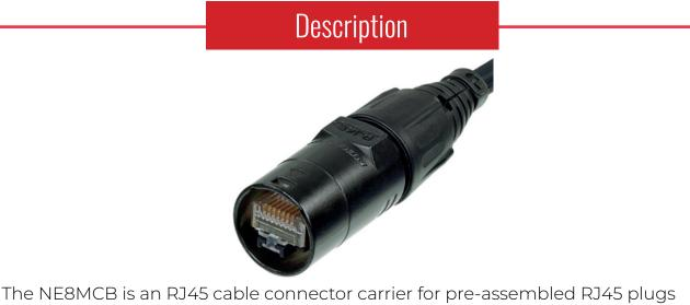
The NE8MCB is an RJ45 cable connector carrier for pre-assembled RJ45 plugs consisting of a black chromium shell, fixing disk, chuck, bushing and boot. Packed with two cable protection elements for cable diameters either up to 5 mm or 8 mm. The cable connector carrier does not include a RJ45 plug.
