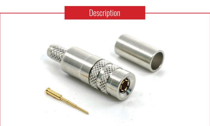
The 1.0/2.3 is a straight full-crimp plug with a gold-plated centre and outer contact with push-pull coupling and a sub-miniature 'true 75 ohm' coaxial connector. Using precision components impedance, it is a re-design of the original DNI style connector, making it suitable for 3G HD-SDI and frequencies up to 12GHz.
